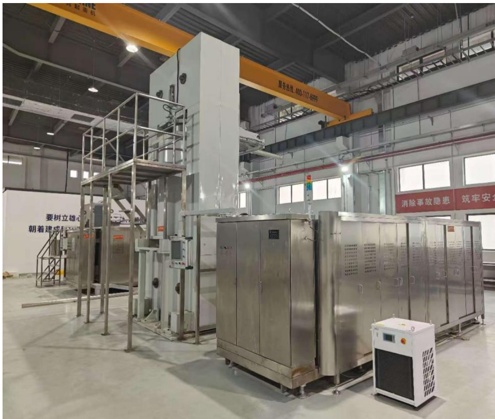
ID400XH600mm and ID800XH1500mm Isostatic Press Machine
